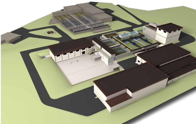
Waterleau's WATERPROOF® compact drinking water plant has been retained by ONEE as best technical and commercial solution. The plant consists of following treatment steps: cascade aeration, optional prechlorination, coagulation, flocculation, decantation, sand filtration and disinfection to ensure a safe and stable drinking water supply. Due to its compact nature, the WATERPROOF® drinking water plant could be constructed using only a minimum footprint.
